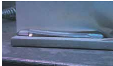
Free peeling slag from a weld made with Select 309L and CO 2 shielding gas.
