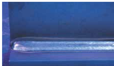
Horizontal fillet produced by Select 308L with CO 2 shielding gas. The bead is even and well-washed, with a finely rippled surface finish.
